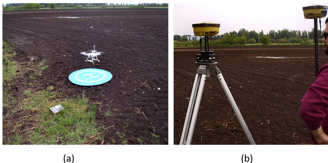
Figure 3. The UAS (a) that collected the RGB imagery and the RTK GPS (b) used to measure GCPs in this study.
