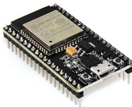
Figure 3. The wireless communication module ESP32 for camera synchronization.
