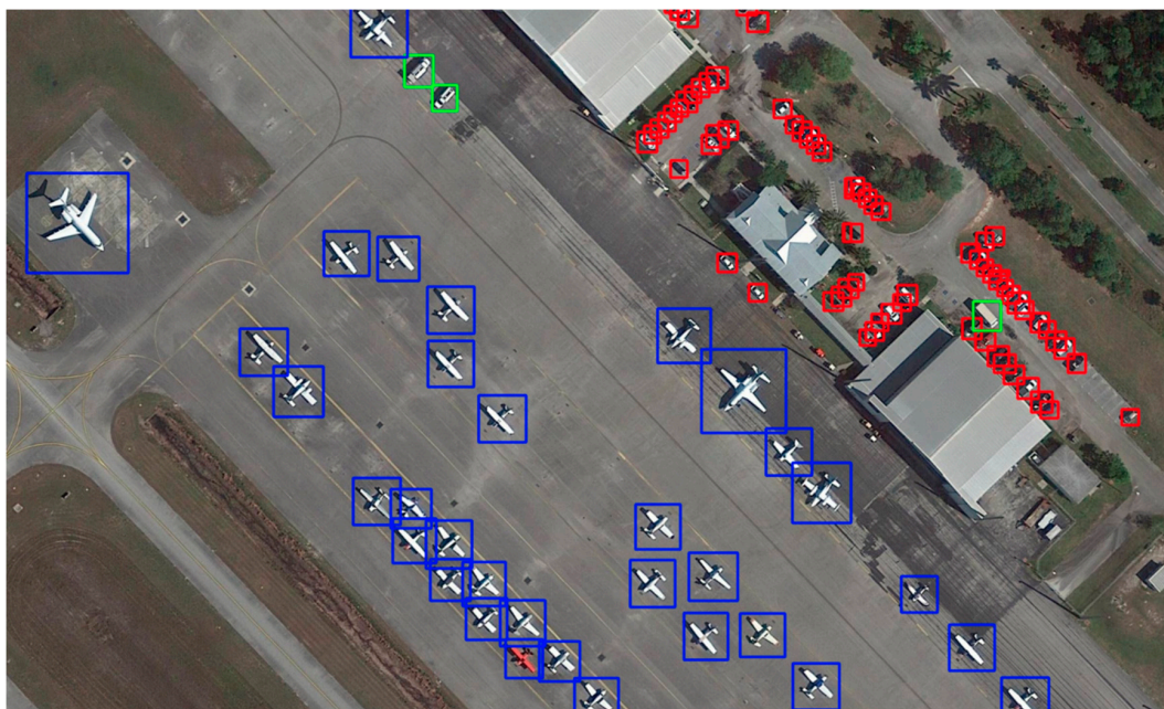
Figure 14. Multi-class geospatial object detection results of MIOU loss-based YOLO v7-Tiny with Truncated NMS in large scenarios on DOTA dataset. The colors of the boxes are the same as Figure 13.
