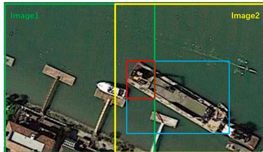
Figure 9. The predicted box filtering in remote sensing images splicing. The red box indicates the predicted box in image1. The blue box is the predicted box in image2.
