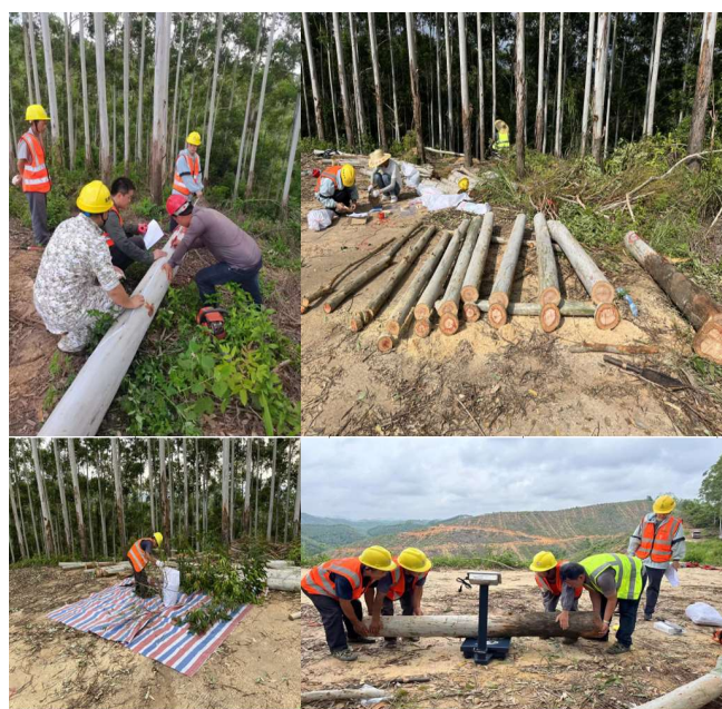
Figure 2. Cutting down of trees and the taking of destructive measurements.
