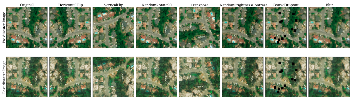
Figure 6. Augmentation techniques were applied to input images for further regularizing the model. On the left, pre- and post-disaster images are displayed, and other images are the outputs of specific augmentations.
