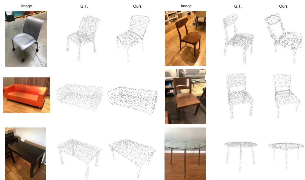
Figure 9. Reconstruction results on Pix3D dataset. For real-world images, our model can still reconstruct complete and accurate point clouds effectively.
