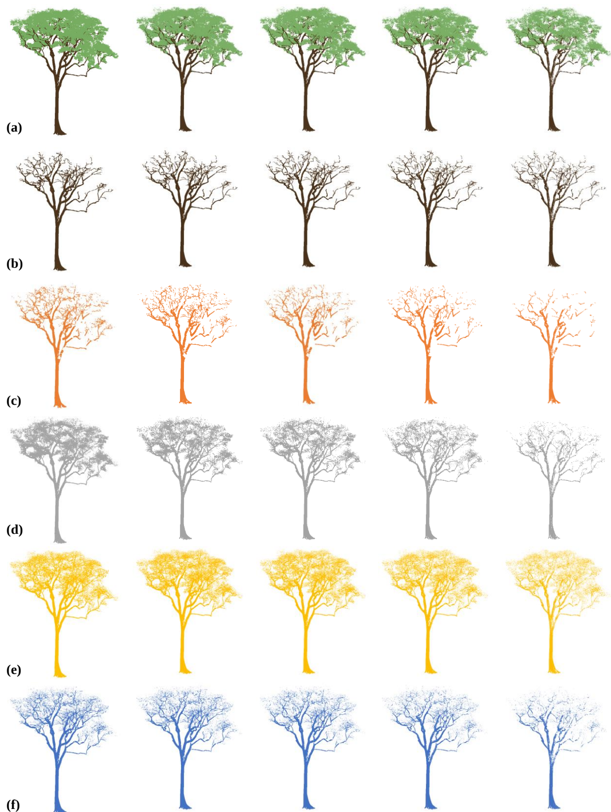
Figure A2. Effect of point cloud subsampling on wood–leaf separation algorithms. Whole tree point cloud (a), manual leaf-filtered point cloud (b), and results of LeWoS (c), TLSeparation (d), CANUPO (e), and RF (f) at different subsampling percentages (unsampled, 30%, 50%, 70%, and 90%).
