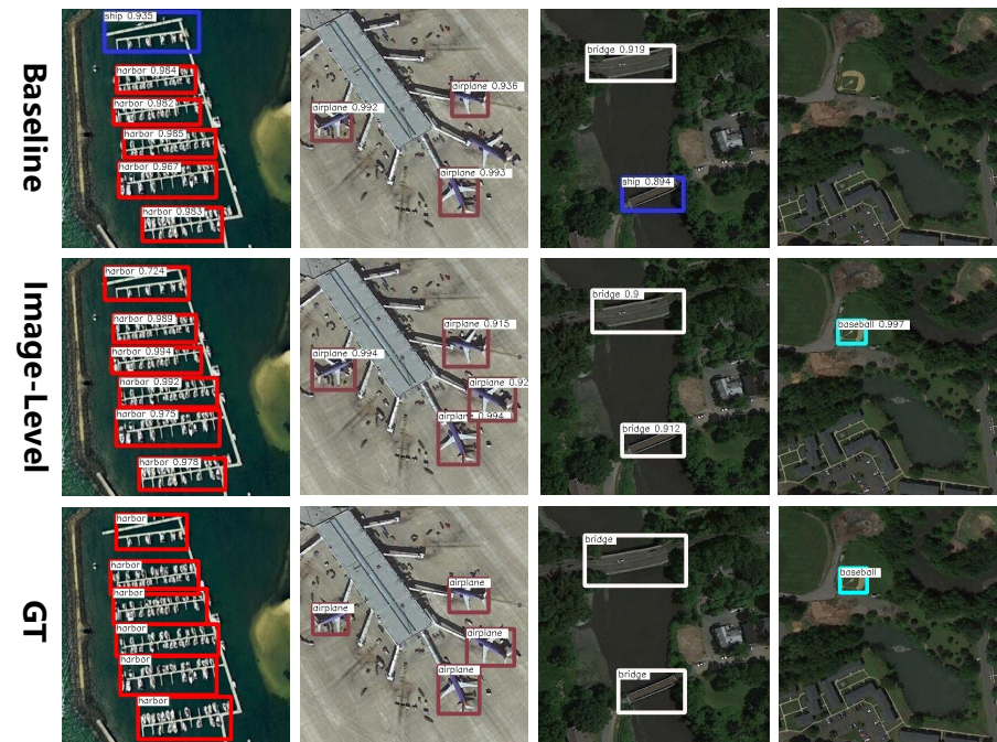
Figure 7. Visualization results of different methods. Compared with the baseline (first row), refining deep features at image level (second row) alleviates the problem of missing detection and reduces the ambiguities in object recognition.
