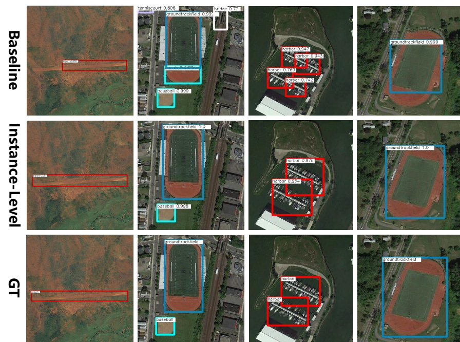
Figure 8. Visualization results of different methods. Compared with the baseline (first row), refining deep features at instance level (second row) alleviates the problem of part domination and has great potential for perceiving the complete instances.
