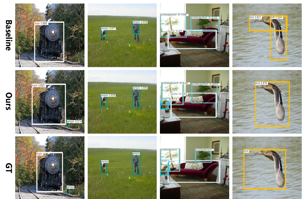
Figure 9. Visualizations of different methods on the VOC2007 dataset. The first row shows the detection results of baseline method and the second row shows the detection results of our proposed method. Taking the third row, visualizations of the ground true, as an indicator, we can clearly see that our method accurately detects the most instances.
