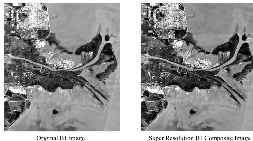
Figure 5. Comparison between the original B1 band and the super-resolution composite band.
