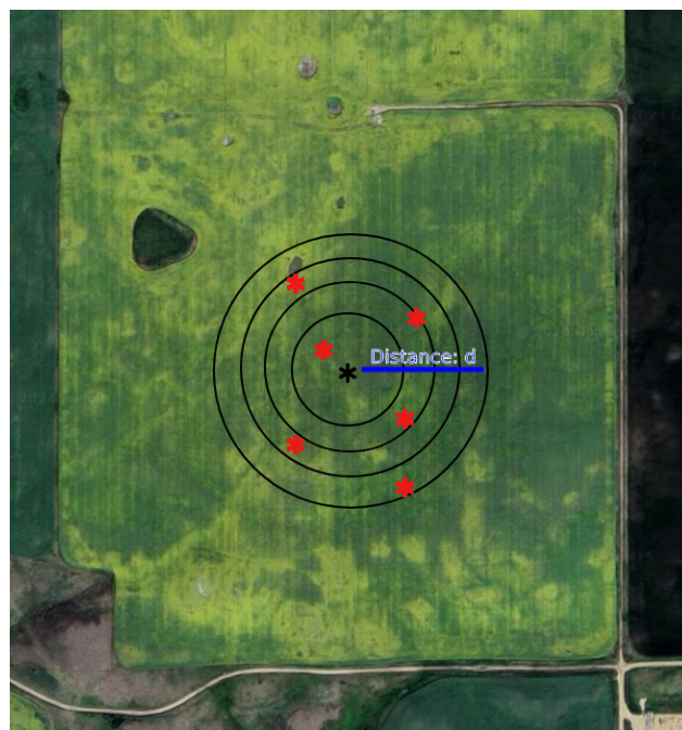
Figure 7. Visualization of sampling method for a field. The black star is the centre of the field and the red stars are the random samples in the area of distance d .
