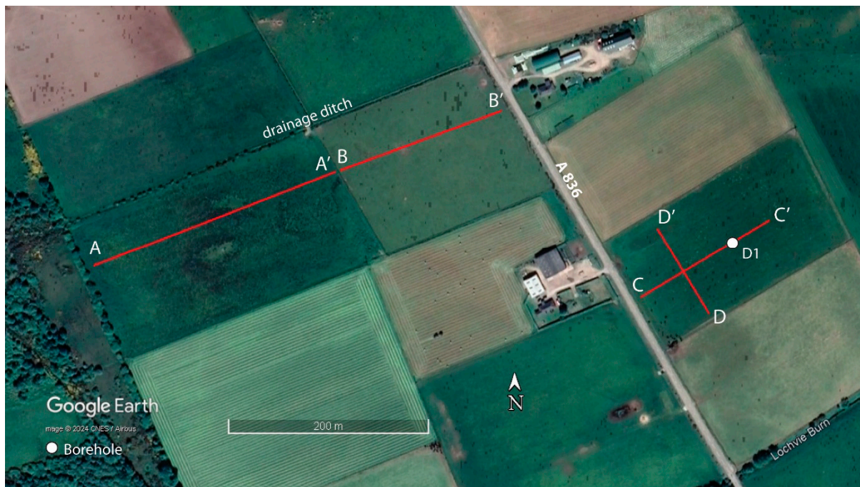
Figure 5. Satellite image showing location of GPR profiles, red lines A-A', B-B', C-C' and D-D', and auger borehole D1 at Dounie.
