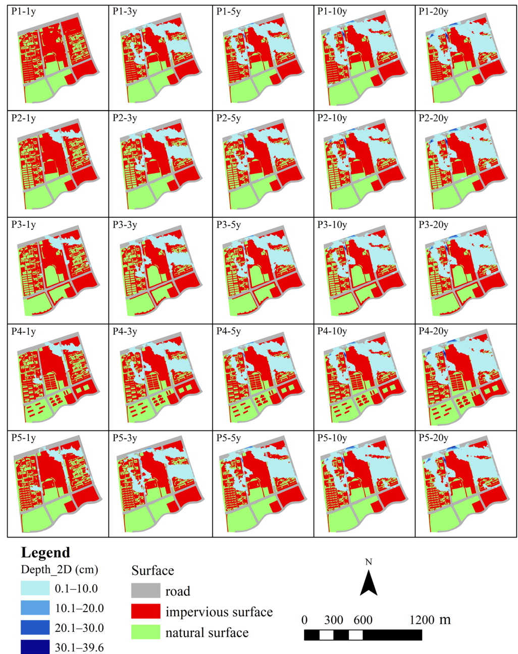
Figure 10. Simulation results of different optimization plans under different return periods: (P1) Land use in 2022; (P2) Impervious surface concentrated upstream; (P3) Impervious surface distributed along roads; (P4) Increase the fragmentation of impervious surfaces; and (P5) Comprehensive distribution.
