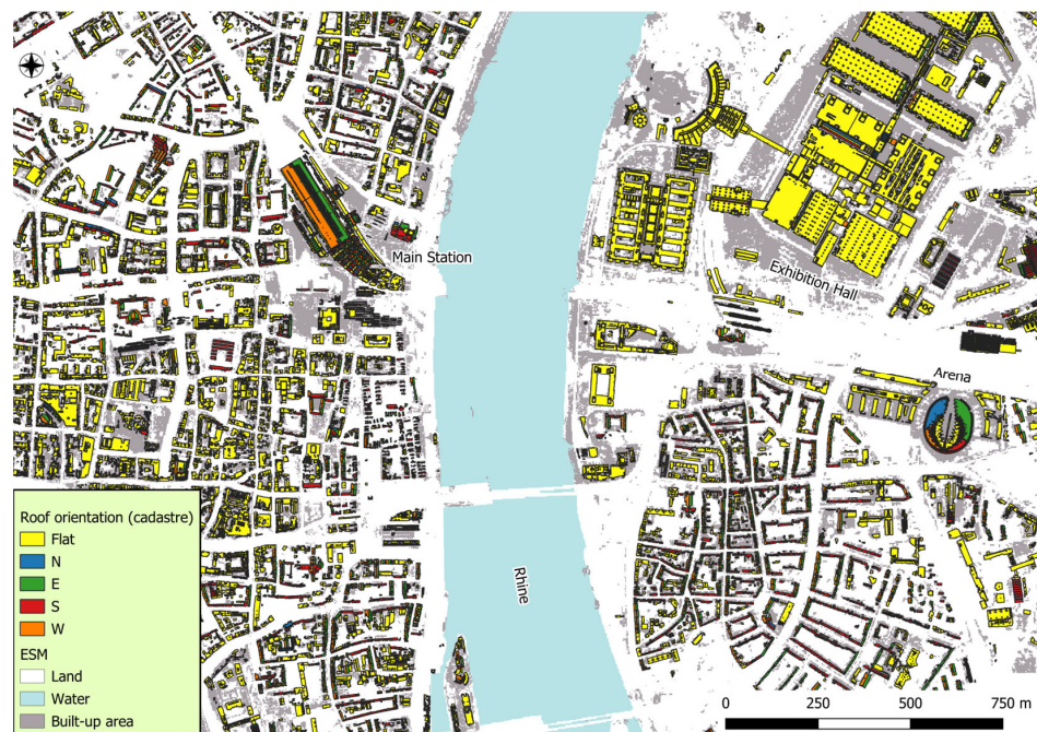
Figure 4. Comparison of European Settlement Map (ESM) [46] estimated built-up area data and roof features and their orientations from the solar cadastre [47] data in the city of Cologne.
