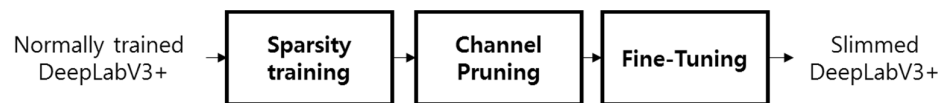
Figure 4. Process of generating a simplified network based on the network slimming method.
