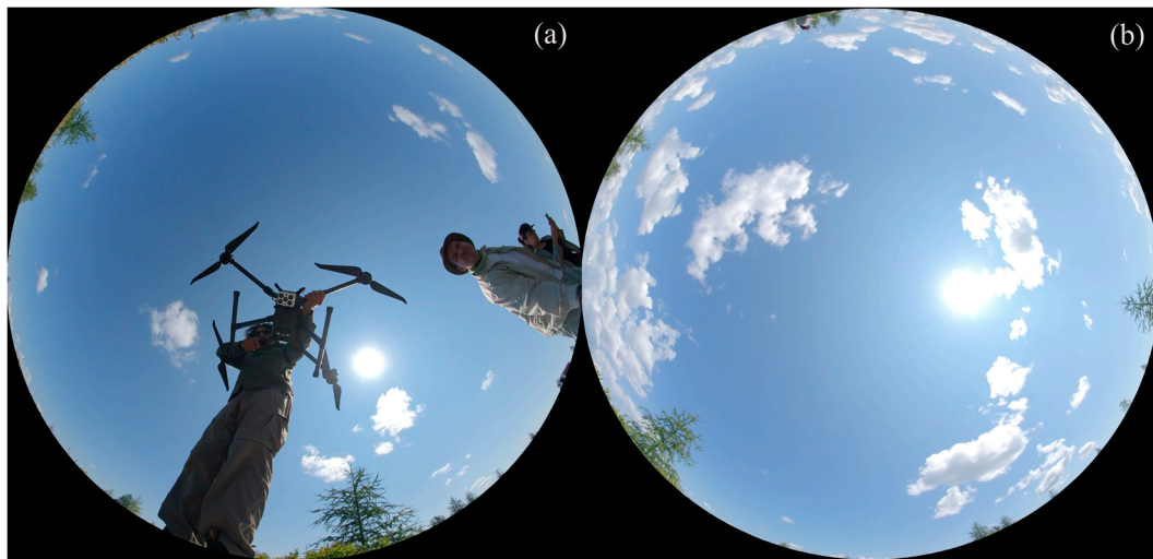
Figure 4. MicaSense recommended calibration procedure captured using an Insta360 camera. (a) Visible obstruction of diffuse irradiance during calibration (excluding the holder of the Insta360 at bottom). (b) Unobstructed sky.
