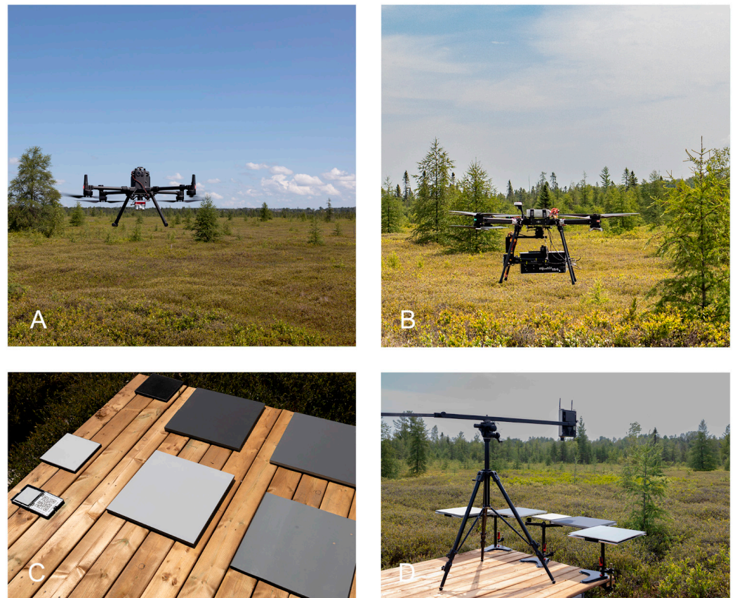
Figure 2. (A) Altum mounted on the M300. (B) Mjolnir VS-620 hyperspectral sensor mounted on an octocopter with a gimbal for stabilization. (C) Six diffuse reflectance panels (2%, 5%, 10%, 18%, 40%, 50%) and the included MicaSense calibration reflectance panel. (D) HR1024i spectroradiometer taking field measurements of diffuse reflectance panels.
