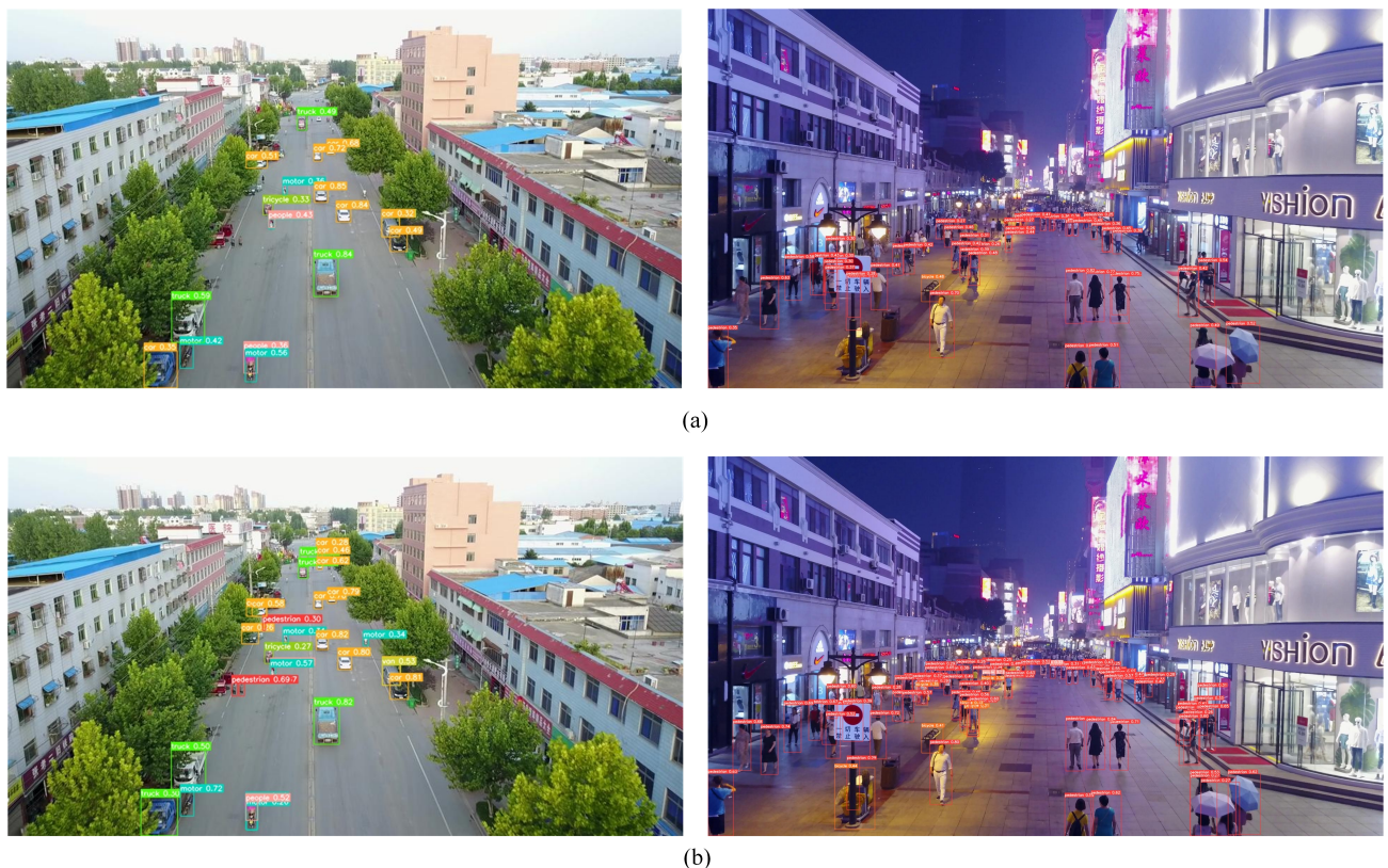
Figure 7. Comparison of detection results on the Visdrone2019 dataset. (a) Based on YOLOv8s. (b) Based on the proposed model.
