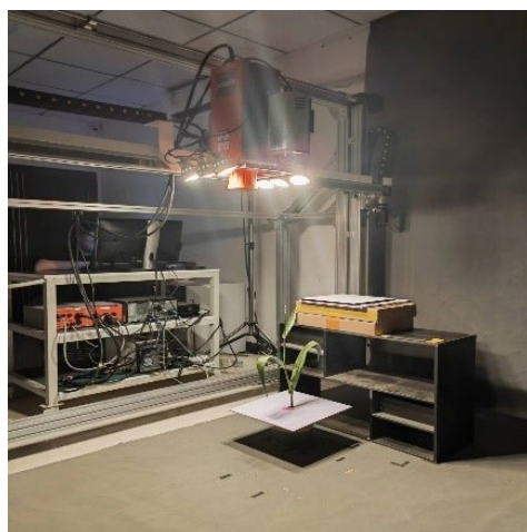
Figure 5. Schematic diagram of darkroom HSI measurement station.
