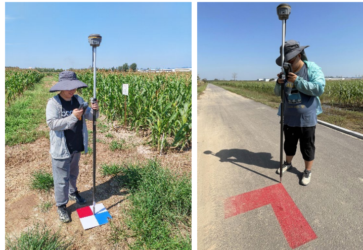
Figure 3. Arrangement of GCP and recording of coordinate information.
