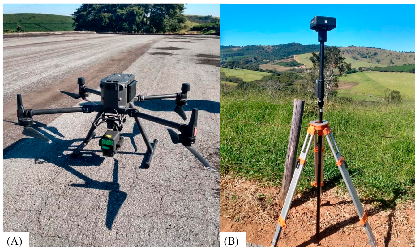
Figure 2. (A) Matrix 300 RTK coupled with Zenmuse L1; (B) DRTK-2 base fixed to the ground.
