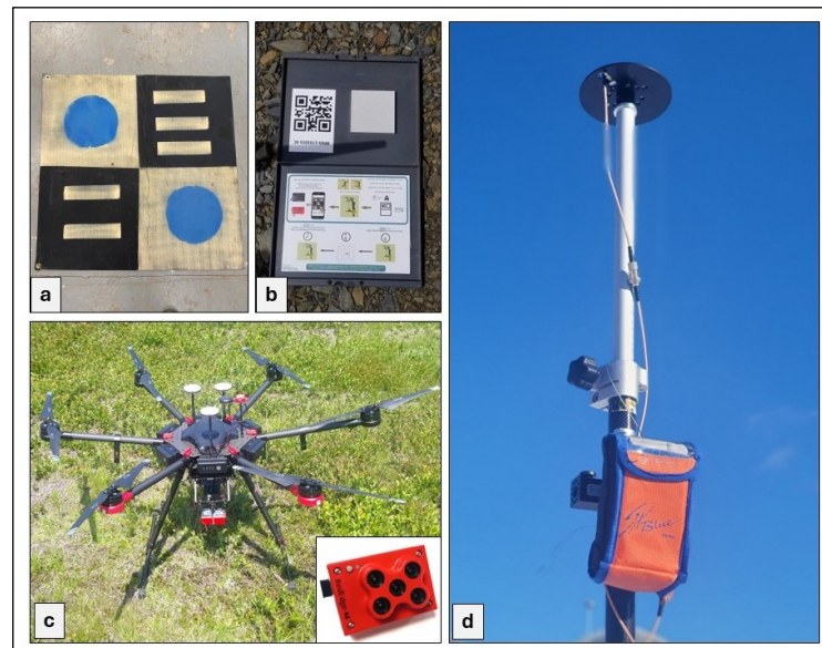
Figure 3. Remote sensing tools. (a) Ground control point, (b) Calibration panel, (c) DJI M600 fitted with an MX multispectral sensor, and (d) SX Blue Platinum GPS device.
