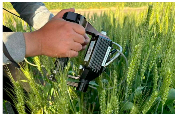
Figure 1. Photograph of non-imaging hyperspectral data acquisition at the leaf scale.
