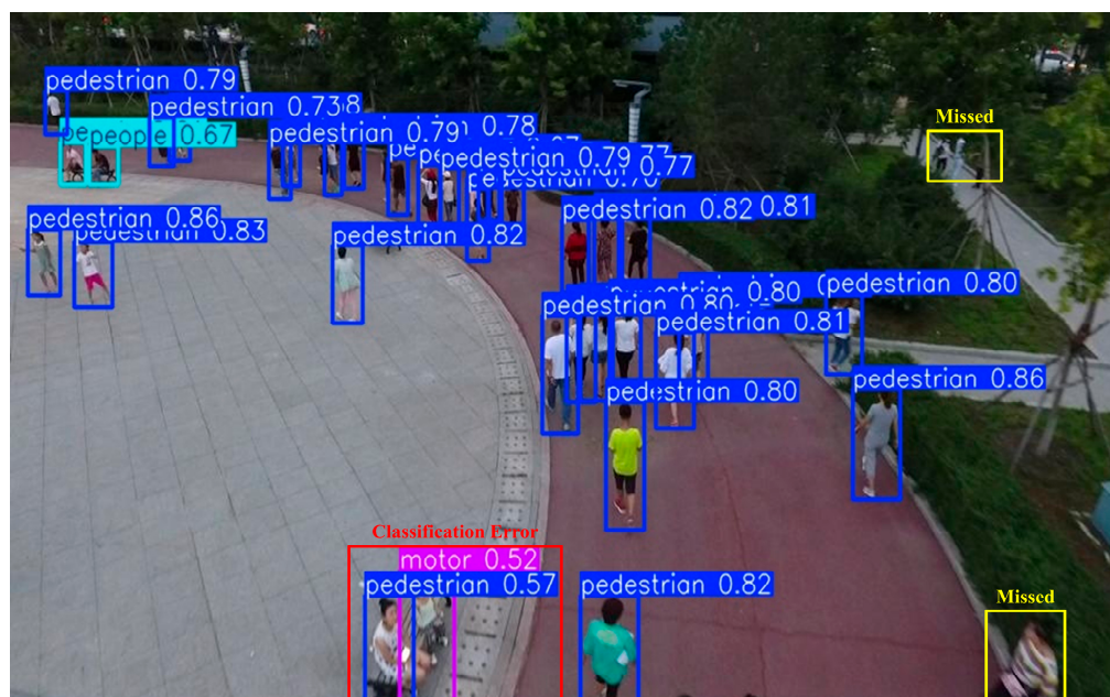
Figure 8. Visualization of typical detection error types. The red box in the figure indicates the classification error results. Two “people” were wrongly predicted as one “motor” and one “pedestrian”. The yellow box indicates the missed detection results.
