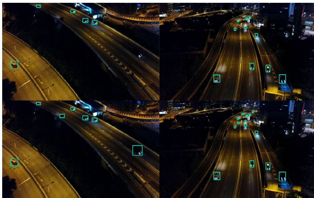
Figure 20. Comparison of detection results of SRTSOD-YOLO-l and YOLO111 in low-light and motion-blurred scenes. The first row shows the prediction results of YOLO111, and the second row shows the prediction results of SRTSOD-YOLO-l. Our model can detect moving blurry targets under low-light conditions.
