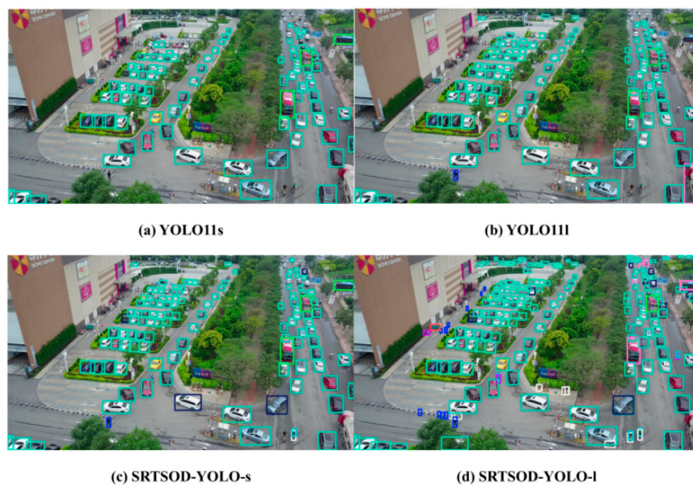
Figure 13. Visualization of experimental results. Boxes of different colors represent targets of different categories predicted by the model.
