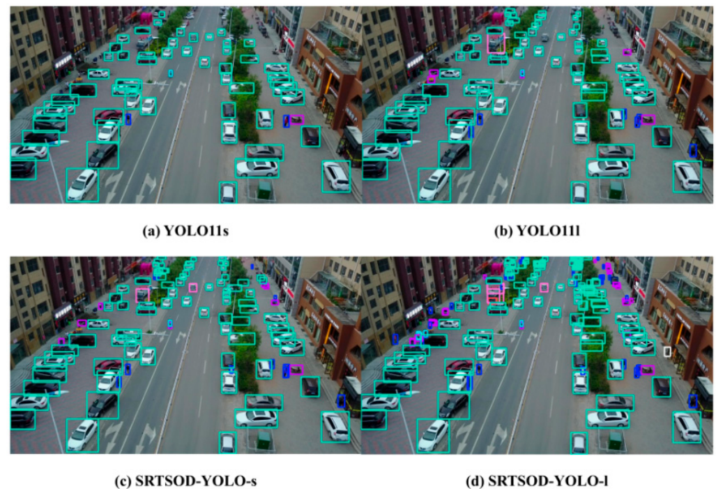
Figure 11. Visualization of experimental results. Boxes of different colors represent targets of different categories predicted by the model.
