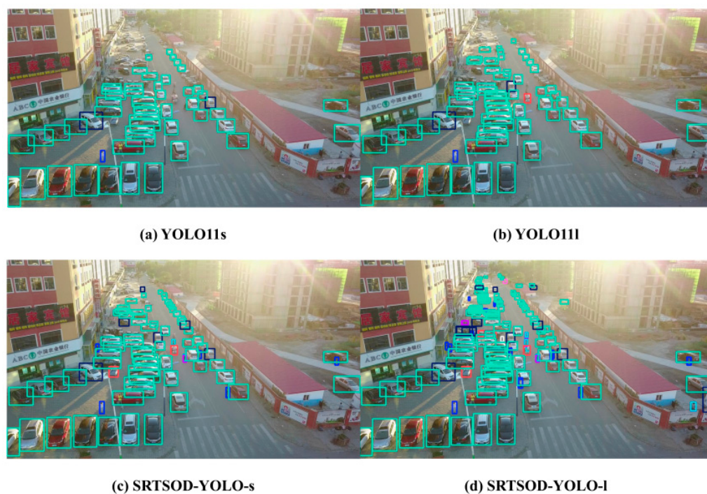
Figure 12. Visualization of experimental results. Our method is capable of detecting small targets that are densely distributed in complex scenarios more effectively. Boxes of different colors represent targets of different categories predicted by the model.
