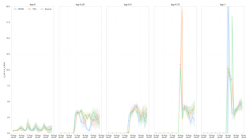
Figure 18. Vertical moment ( z_{cm} + \sigma_z ) of the tracer column along the transect for tr17_t2 (legs 0, 0.25, 0.5, 0.75, and 1). The curves indicating MYNN, YSU, and BouLac.
