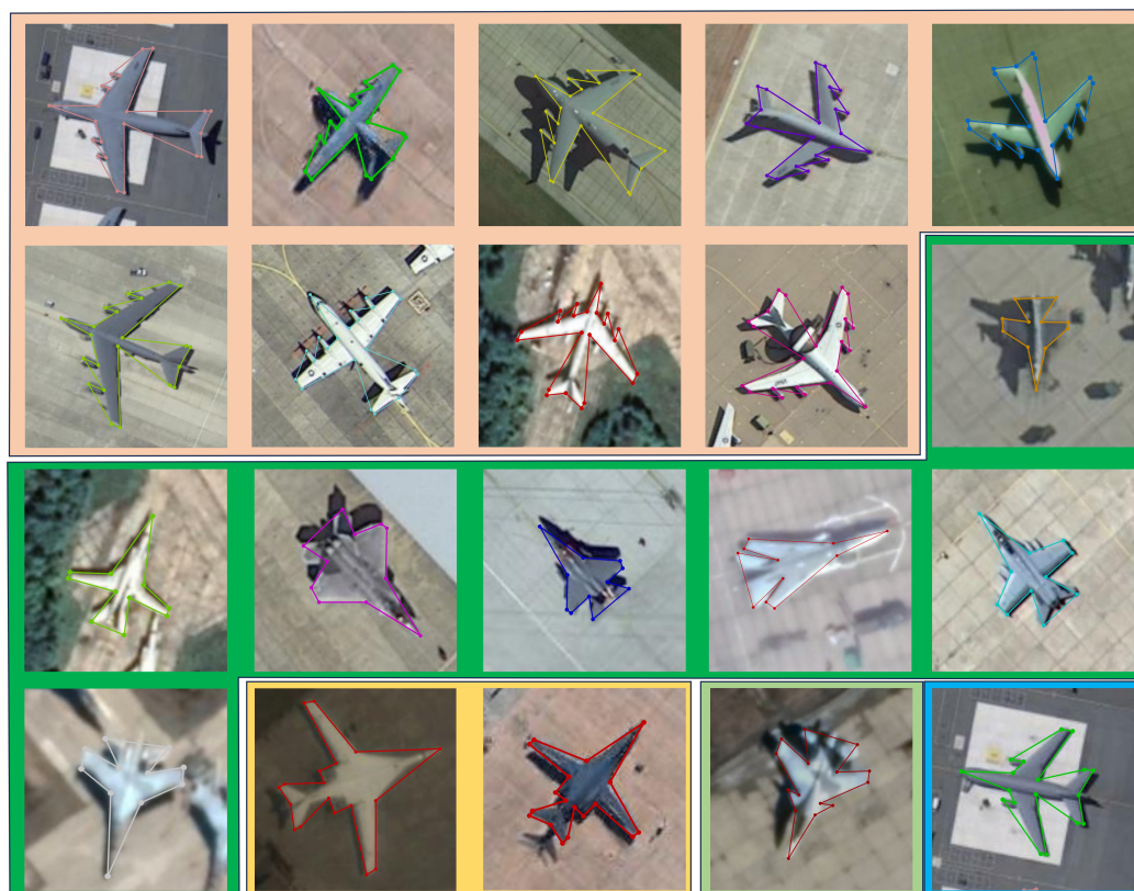
Figure 4. Samples in the keypoint dataset. Five colors indicates five types of aircraft, each type of which shares similar design. Different colored lines are polygon annotation of different aircraft.
