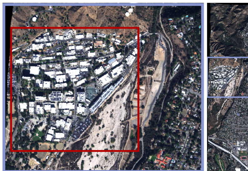
Figure 1. On the right: image of the AVIRIS-NG flightline ang20171108t184829, constructed by taking the red, green, and blue channels from the hyperspectral image. The site over which the larger-scale retrieval was performed is shown in the left part of the figure, outlined by the red rectangle. The zoomed-in part is marked by the blue rectangle in the zoomed-out image of the flightline. The site chosen for the retrieval includes the Jet Propulsion Laboratory in Pasadena, California, and consists of 160,000 pixels. The scene is heterogeneous and includes both built-up and more natural sections.
