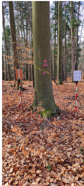
Figure 3. An individual tree ready for photogrammetric data collection (the photogrammetric marker followed the standard Agisoft design and was exported directly from Agisoft Metashape.).
