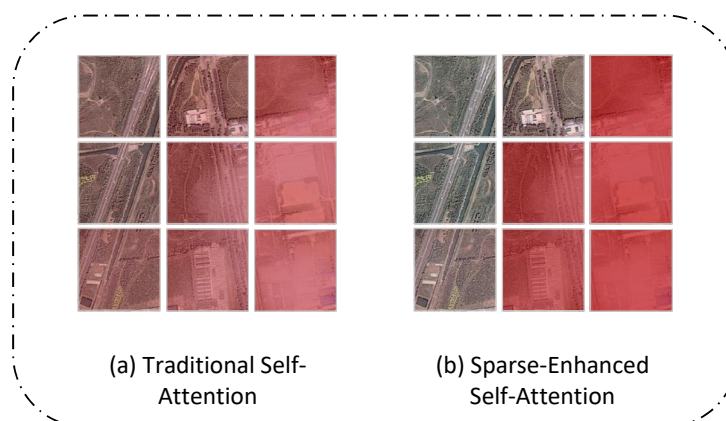
Figure 3. The difference between traditional Self-Attention and Sparse-Enhanced Self-Attention. The Sparse-Enhanced Self-Attention module applies localized enhancement and suppression to the traditional Self-Attention mechanism.
