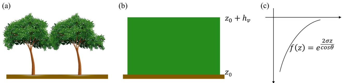
Figure 3. RVoG model for sub-canopy topography retrieval using InSAR. (a) Forest scenario; (b) Forest volume medium modeled by RVoG model; (c) Vertical structure function. In (b), the forest structure is modeled as a two-layer scattering volume, where z_0 denotes the ground elevation and z_0 + h_v represents the height of the scattering volume. f(z) indicates the radar reflectivity at different scattering heights, whose attenuation is governed by the extinction coefficient \sigma .
