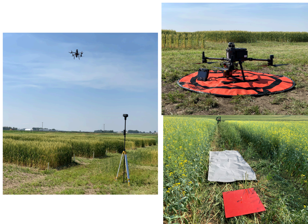
Figure 2. Representative photographs illustrating key steps of data collection conducted during the study: (top right) UAV equipped with MSI/HSI sensors prior to flight operations; (bottom right) calibration tarp used for radiometric calibration of HSI imagery; and (left) UAV flying over crop plots equipped with the DJI D-RTK 2 system.
