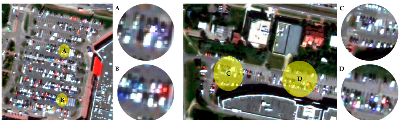
Figure 5. Challenges in vehicle detection in satellite data (WorldView-2, GSD = 0.5, Central Europe): shadows, occlusion by trees, low contrast, and reflection artifacts for bright objects. Yellow circles indicate selected regions of interest, while capital letters (A–D) link these regions to the corresponding enlarged examples shown next to the satellite images.
