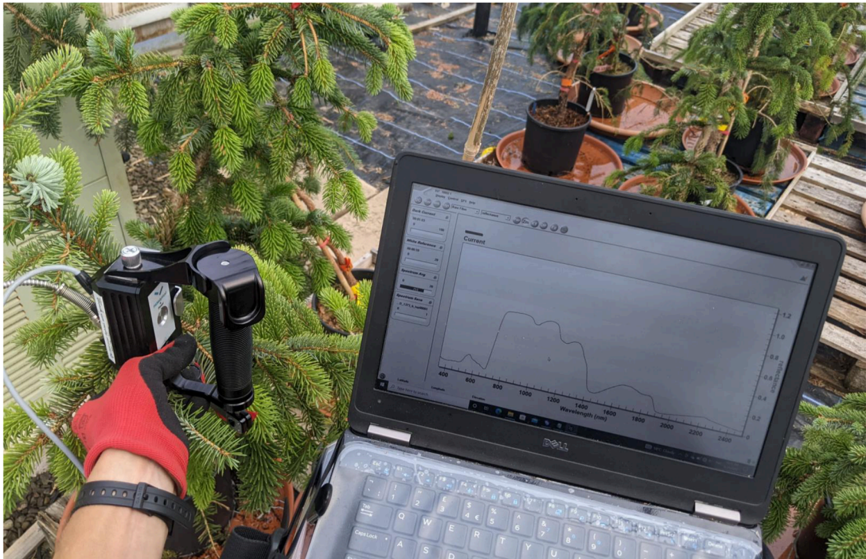
Figure 1. Needle-level hyperspectral measurements acquired from Sitka spruce ( Picea sitchensis ) using an ASD FieldSpec 4 spectroradiometer fitted with a contact probe. Reflectance measurements were collected repeatedly throughout the drought experiment to monitor temporal changes in physiological status under control and drought treatments.
