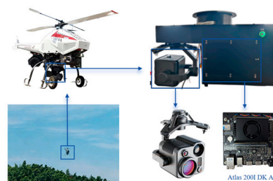
Figure 16. M 2 CA-FFM algorithm, UAV-based inference, and verification system.
