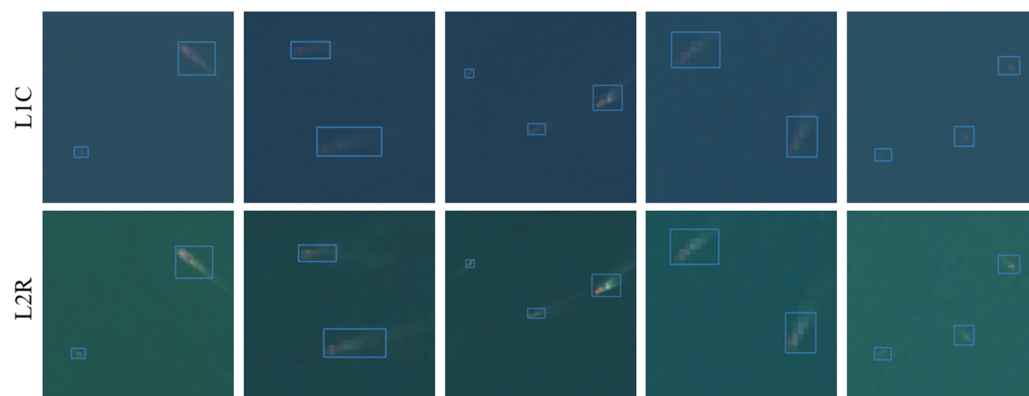
Figure 2. Visual comparison of manual vessel annotations between original TOA reflectance (L1C, top row ) and ACOLITE-corrected surface reflectance (L2R, bottom row ), with blue boxes highlighting the annotated targets.
