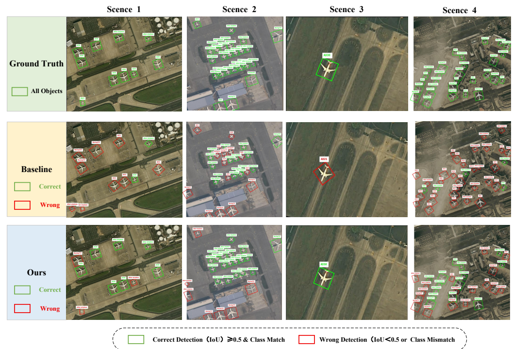
Figure 12. Qualitative detection results on test images. Green bounding boxes denote correct detections ( \text{IoU} \geq 0.5 and accurate classification), while red boxes indicate incorrect detections (localization error or class mismatch). Compared with the baseline methods, the proposed method achieves higher detection accuracy.
