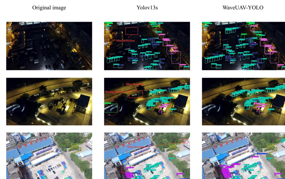
Figure 12. Qualitative detection results comparison in extreme environments, detailing the predictions of the baseline YOLOv13s (middle column) and our proposed WaveUAV-YOLO (right column).
