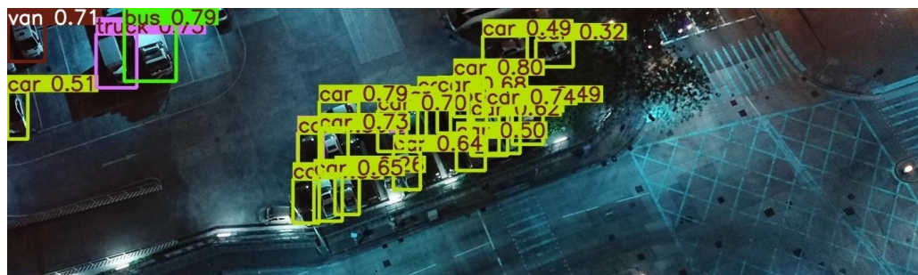
Figure 15. Visualization of a typical failure case in an extremely dense and shadowed environment. The model occasionally exhibits missed detections (false negatives) in heavy shadows where edge gradients decay and redundant bounding boxes (false positives) triggered by complex reflections and high-frequency noise interference.
