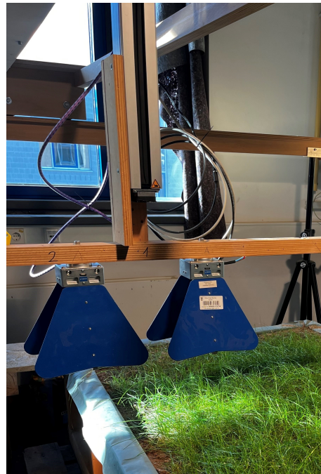
Figure 1. The antennas (blue) are mounted on the axis of the cross table above the grass test area.
