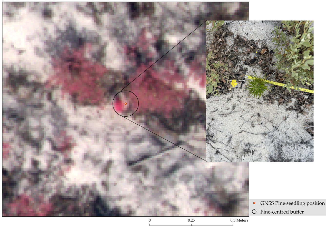
Figure 8. Example of pine-centred buffer construction for an individual Pinus pinaster seedling. The GNSS seedling position is shown over the multispectral orthomosaic, together with the corresponding buffer derived from the measured crown dimensions and additional radial margin. The inset shows the field photograph of the same seedling.
