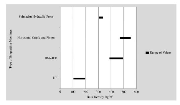
Figure 6. Ranges of the bulk densities of the different briquette molders developed.
