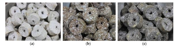
**Figure 5.** Types of briquettes produced using biomass wastes, from left to right: (a) paper (P); (b) paper + sawdust (P + SD); and (c) paper + sawdust + carbonized rice husk (CRH) (P + SD + CRH).
