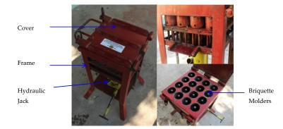
Figure 1. The hydraulic jack-driven briquetting machine utilized in the briquette production test.
