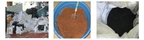
**Figure 3.** The materials used in briquette production, namely, from left to right: waste paper, sawdust and carbonized rice husk.
