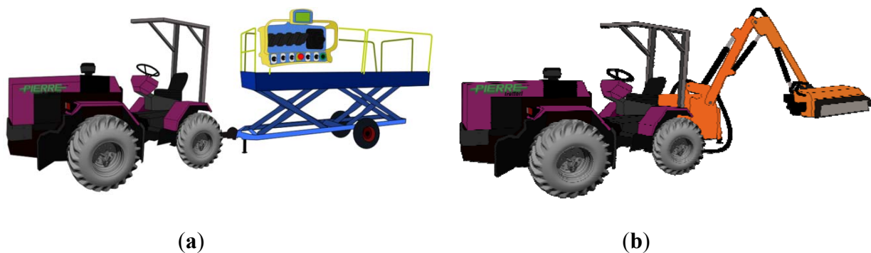
Figure 9. Example applications of the tractor with TECS: (a) with orchard platform; (b) with side-arm brushcutter.
