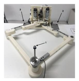
Figure 20. Placement of the markers on the prototype for the experimental procedure.
