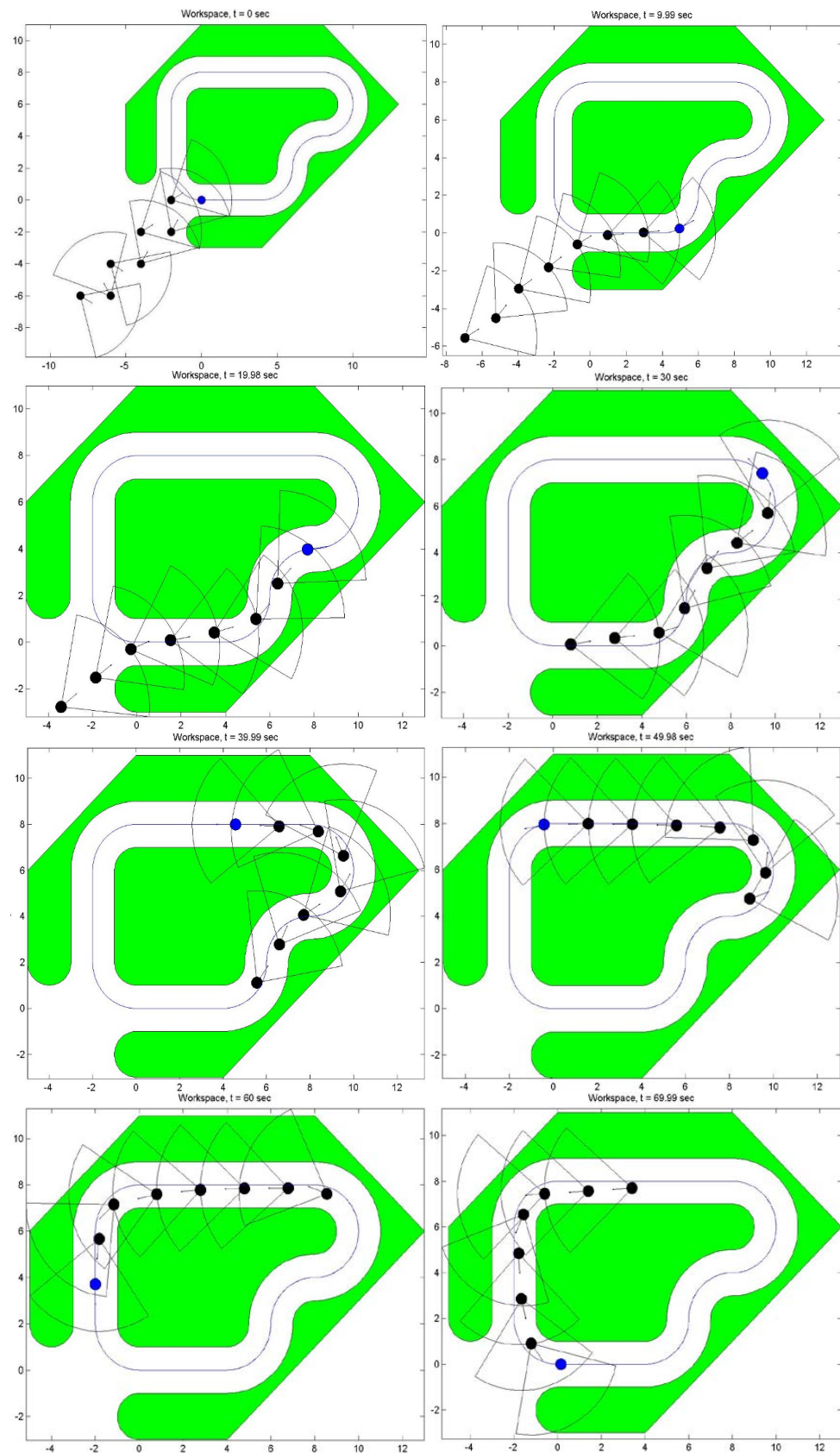
Figure 5. Study A: The operation of the robot-team (blue color indicates the leading robot and black the following ones) is depicted for 8 consecutive time instants, every 10 s. Each camera field of view is given by the black quadrants.
