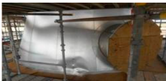
Damage to brine concentrator—post-impact.
