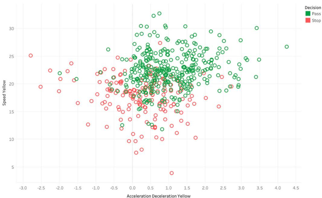
Figure 6. Correlation of driver’s decision with speed and acceleration/deceleration.
