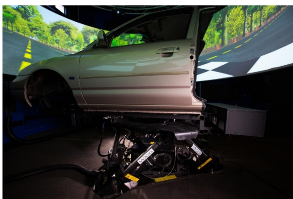
Figure 4. Simulator (motion platform).
