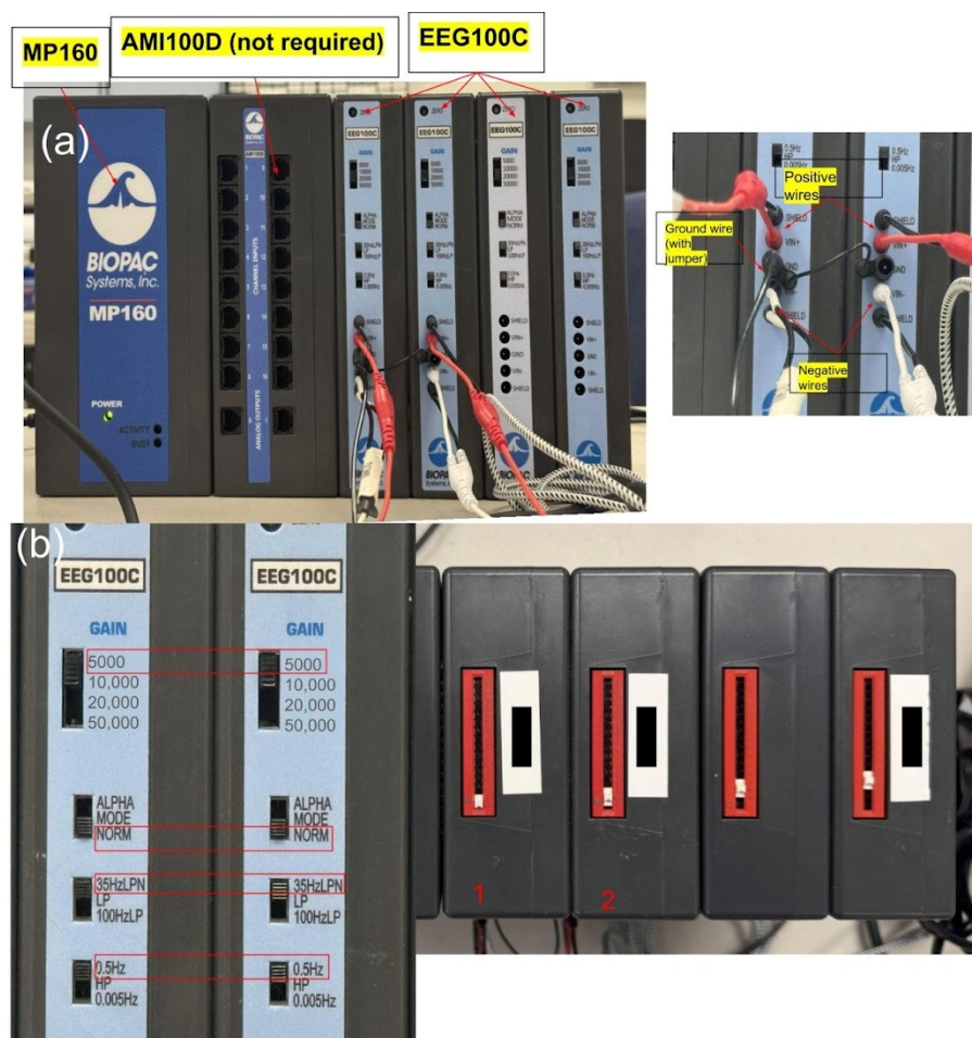
Figure 3. (a) BIOPAC® acquisition system setup to measure EMG signals. (b) Settings on amplifiers. Only amplifiers 1 and 2 were needed to measure the left and right upper trapezius regions.
