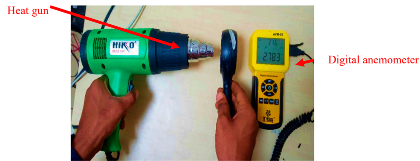
Figure 1. Flow rate measurement of hot air using Digital Anemometer.
