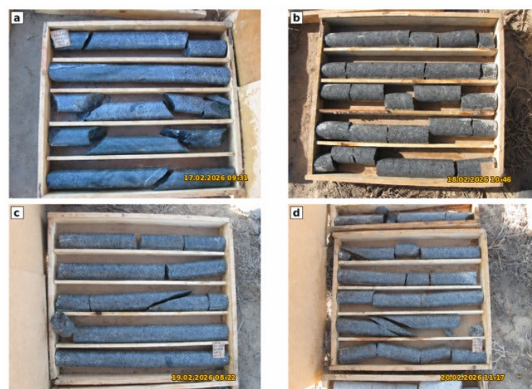
Figure 2. Representative geotechnical core conditions: (a) relatively intact core with isolated breaks; (b) moderately fragmented core; (c,d) core containing inclined natural discontinuities.
