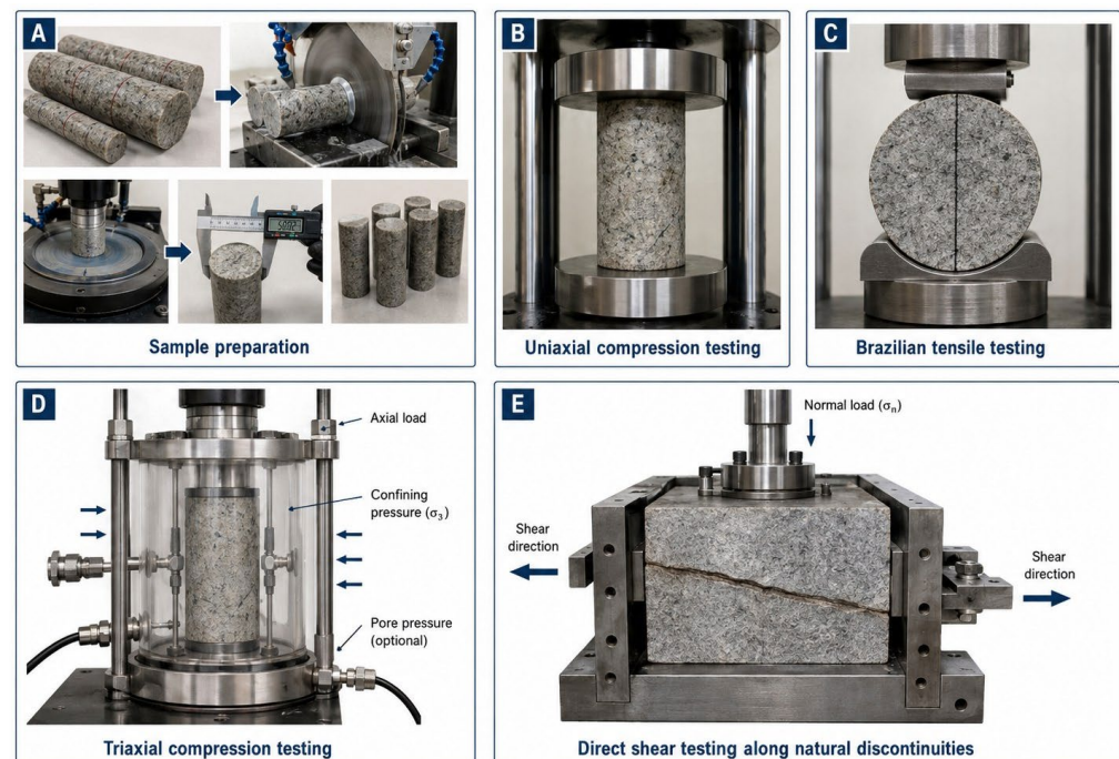
Figure 3. Schematic representation of the laboratory tests: (A) specimen preparation; (B) uniaxial compression; (C) Brazilian tensile test; (D) triaxial compression; (E) direct shear along a natural discontinuity.
