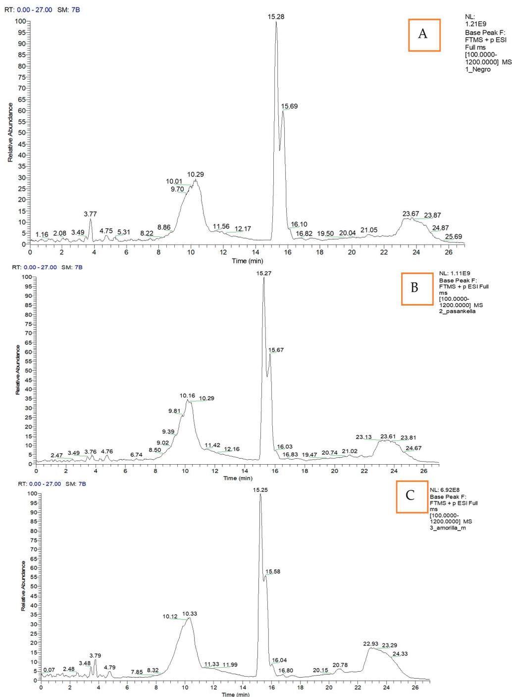
**Figure 3.** Chromatographic profile (LC-MS) of the hydroalcoholic extract of *C. quinoa* sprouts. (A) Black coito, Rt (min)—15.28, betaine; 15.69, choline. (B) Pasankalla, Rt (min)—15.27, valine. (C) Yellow maranganí, Rt (min)—15.25, betaine; 15.58, choline in ESI (+) ionization mode.
