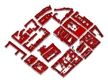
**Figure 11.** Model of a historical city determined by the proposed, data driven approach. The roofscape is shown in red and vertical walls in gray.
