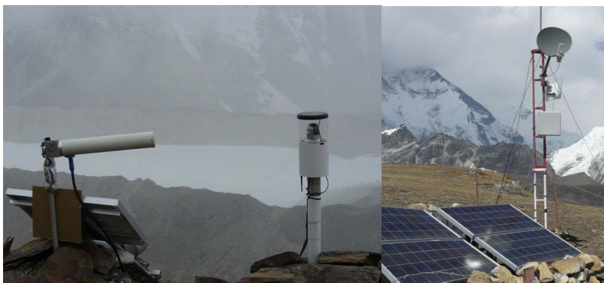
Figure 9. Fieldservers and wireless relay station for monitoring Imja Lake (Altitude: 5,000 m).
