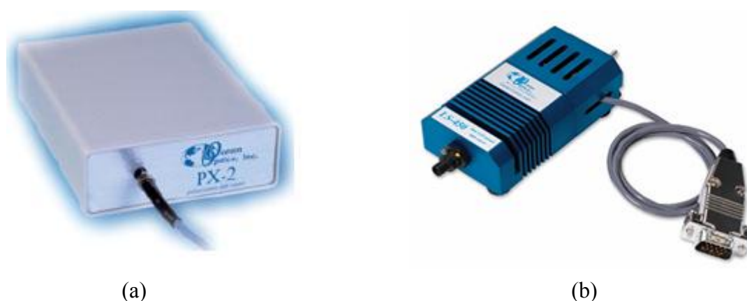
Figure 4. Two excitation light sources were considered for the real-time PCR on-chip system: (a) shows the white light lamp with light-intensity control ability to 3% variation, and (b) shows the LED providing a simple excitation light source with high intensity variation to 5%.
